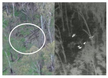
Figure 10. Thermal video cameras fitted to helicopters or drones can clearly and quickly detect feral deer in dense vegetation (right), compared with the ability of the human eye (left, circle). Photo from HeliSurveys (website).
